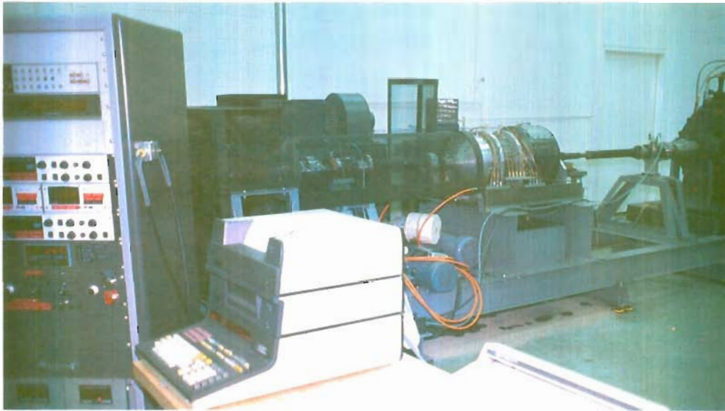
Bench testing of Vadetec CVT prototypes depends upon a 9830 desktop computer for control of data acquisition and processing. Vadetec plans to modify the system further in the near future to control the entire test process.
