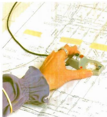
Digitizing has made it possible to phase out 'scissors drafting' methods of maintaining extensive gas company tract maps.
